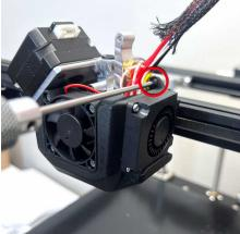
• Install the assembled fan shroud back onto the extruder using two M3 screws. (2.0mm Allen Wrench)
