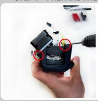
• Prepare the NG Revo Extruder by removing the two screws holding the fan shroud.
