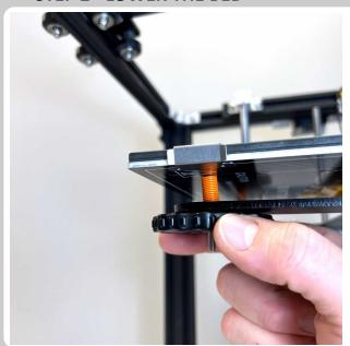
The position of the nozzle and probe will be at a slightly different height, so doing this step will prevent the nozzle from crashing into the bed.
