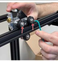
• Insert the provided shorter M5 screws into the two remaining V-Roller wheels.
