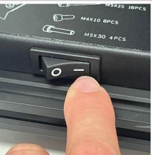
Plug the power cable in and turn the printer on
