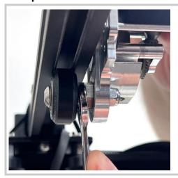
To eliminate any wobble from the carriage, adjust the tension of the V-Roller wheels by rotating the eccentric nut using a 10mm wrench
