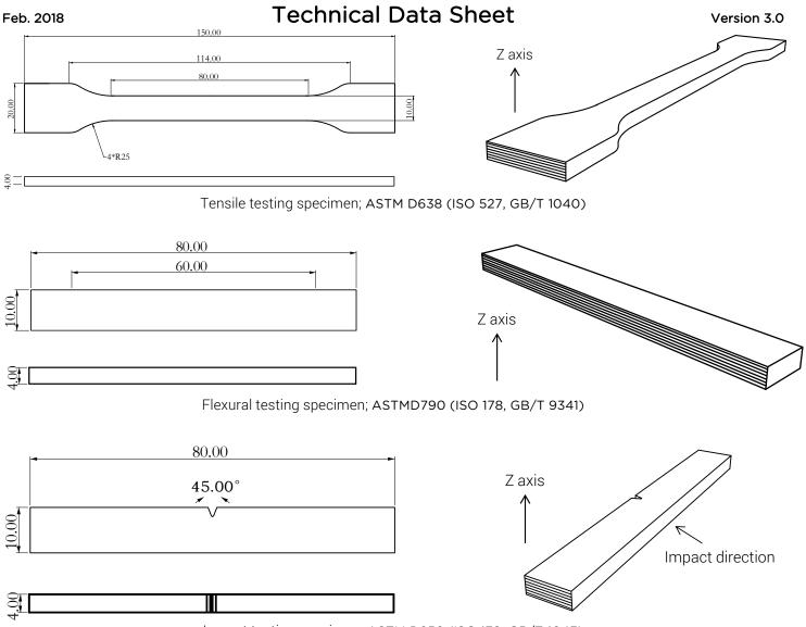
Impact testing specimen; ASTM D256 (ISO 179, GB/T 1043)
