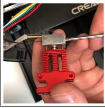
With provided 1.5mm allen wrench, unscrew both setscrews that hold the heater cartridge and the thermistor
