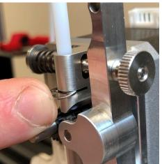
Insert the filament guide tube and secure it with the provided retaining clip
