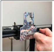
Use provided (2x) M4x16mm screws to mount the cartridge on the ExoSlide block
