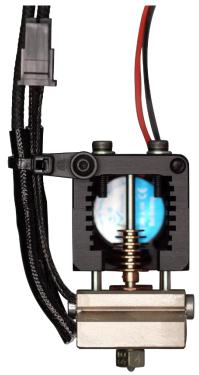
Figure 13. Mosquito<sup>™</sup> with temperature sensor, heater cartridge, fan, and nozzle installed with strain relief.
