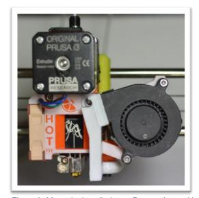
Figure 9. Mosquito installed on a Prusa printer with the Noctua fan that comes with the Prusa
