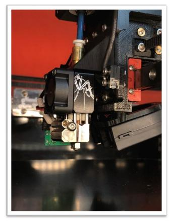
Figure 11. Mosquito™ with fan installed
